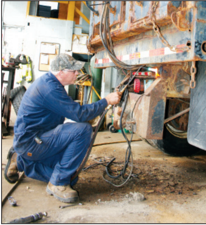
Highway Department mechanic Bob Adams works on removing the large sander dump body from the department's heavy duty 1994 six-wheel Brigadier truck, in preparation for that to be replaced by a newer stainless steel model.
