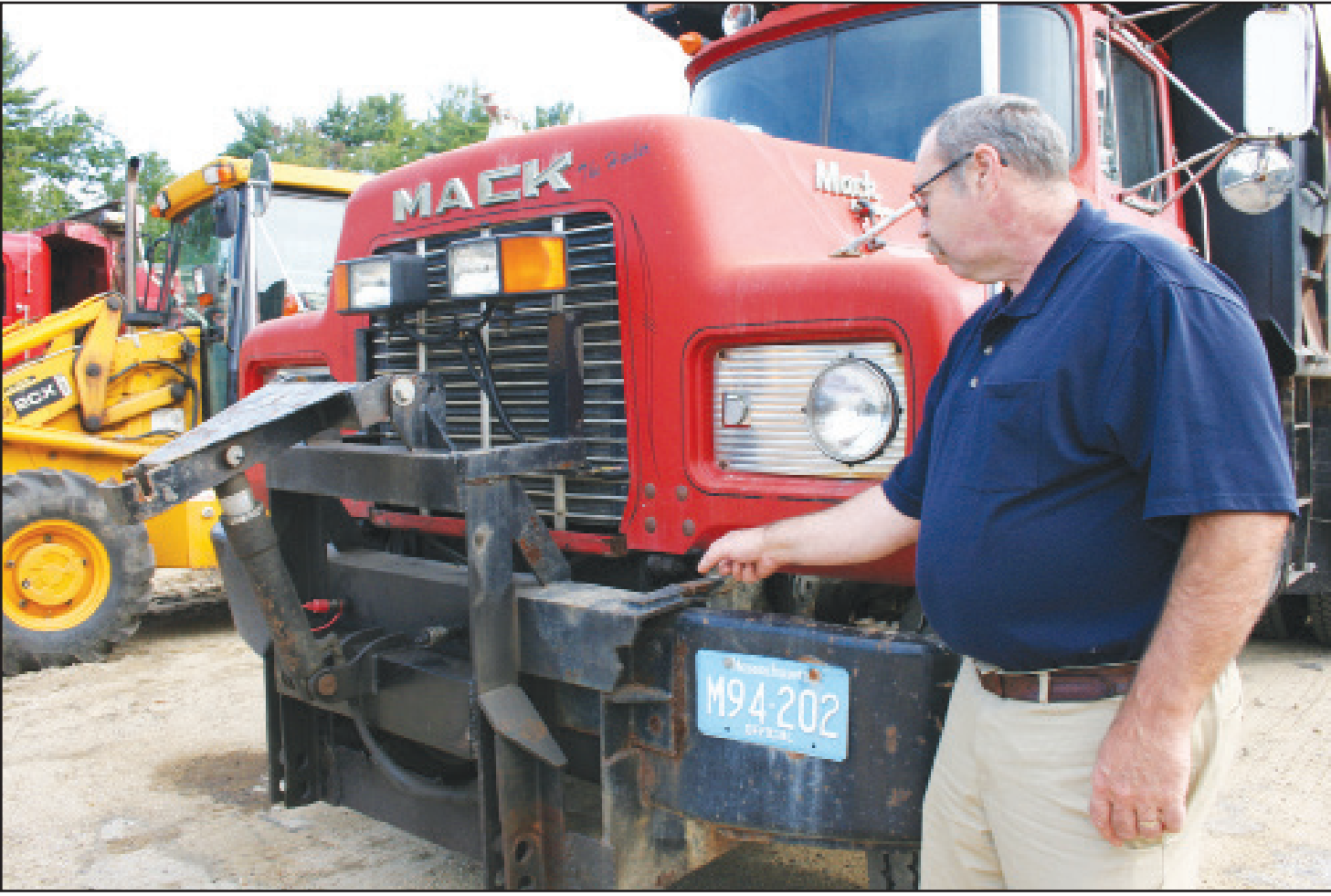
Public Works Director Alan Mayo points out where a crack has formed in the front frame of the bumper on the department's 1984 Mack 10-wheeler truck which is used for attaching a plow onto the vehicle.
